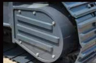
Rear of travel motor cover is reinforced.
