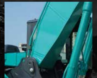
Newly designed, big cross-section boom for unbeatable durability under harsh working conditions.
