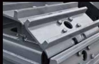
The double grouser shoe consisting of a thick plate and having a strong grip force and sufficient strength is also selectable. This is proper for severe working conditions in mining sites.
