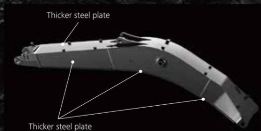
The XD boom features stronger plates compared to the HD booms of standard machines, which increases longevity even under the toughest working conditions.
