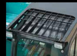
The top guard (FOPS, Top Guard Level II. (Meets ISO10262)) provided as standard. The top-mounted working light ensures a wide field of view.
