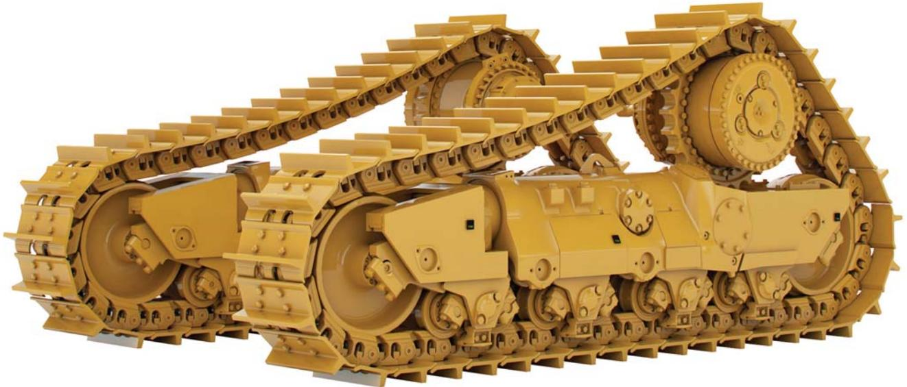
The elevated sprocket and fully suspended undercarriage work together, increasing traction while creating a smoother ride for your operators. The elevated sprocket design transfers implement shock loads to the mainframe, so final drives, axles and steering components are isolated from harsh impacts. These benefits translate into higher production and longer component life.
