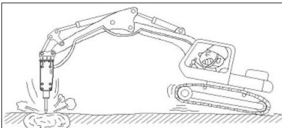
It is undesirable to carry out hammering under the below condition, because vibrations during hammering may be transmitted to the tracks of the base machine. During hammering, however, proper position must be always applied to the breaker. Special care must be taken not to hammer under abnormal condition.
