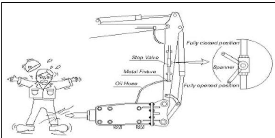
3) Loosen the hose plug on the breaker arm
