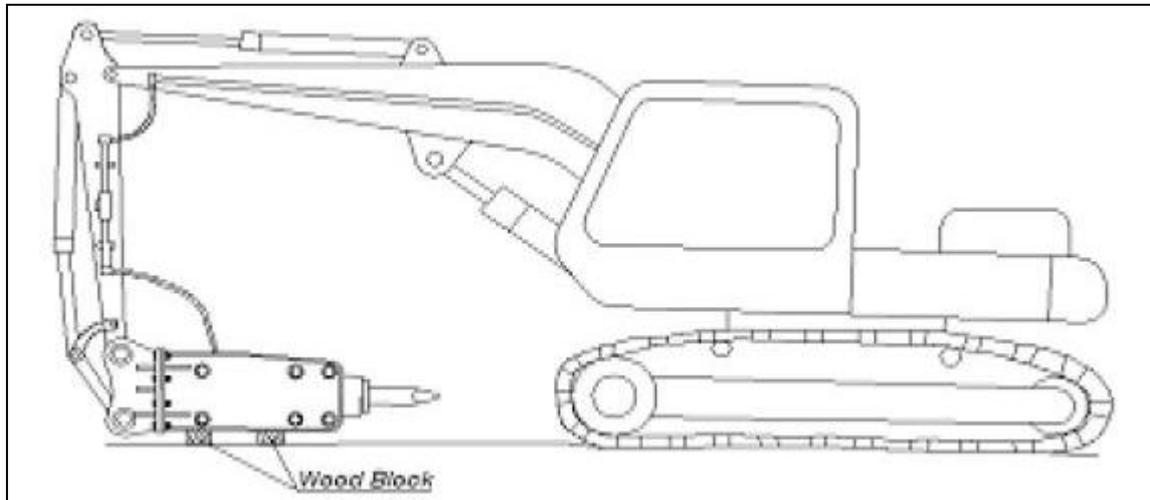
2) Turn the shut off valve (installed to the end of the boom arm) 90 degrees to the "off" position to prevent the hydraulic oil from flowing out.
