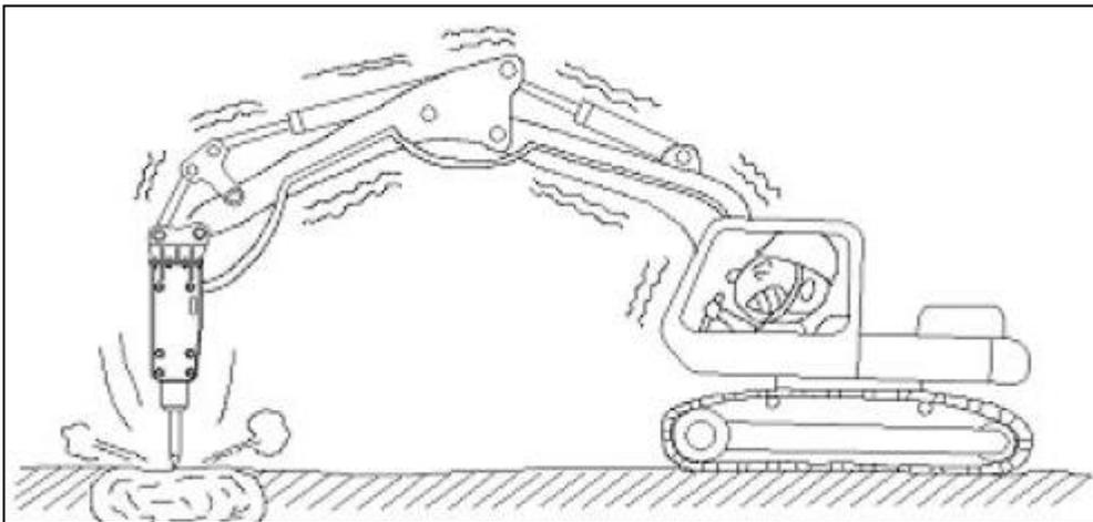
On the contrary, when position is excessive enough to break rocks with the front of the base machine raised, the machine may suddenly tilt forward the moment rocks are broken. Then, the breaker body or the end of bracket may violently hit against rocks and result in damage.
