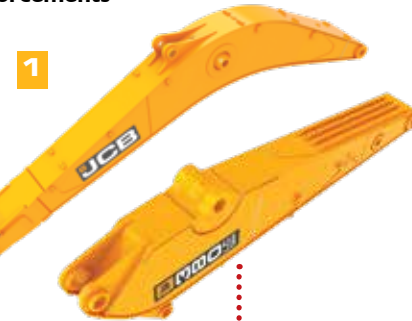
Heavy duty boom & arm with reinforcements
