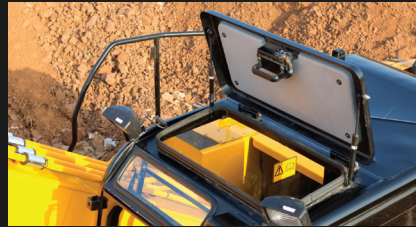
Easy to open roof hatch assisted helps to keep the cab well ventilated.
