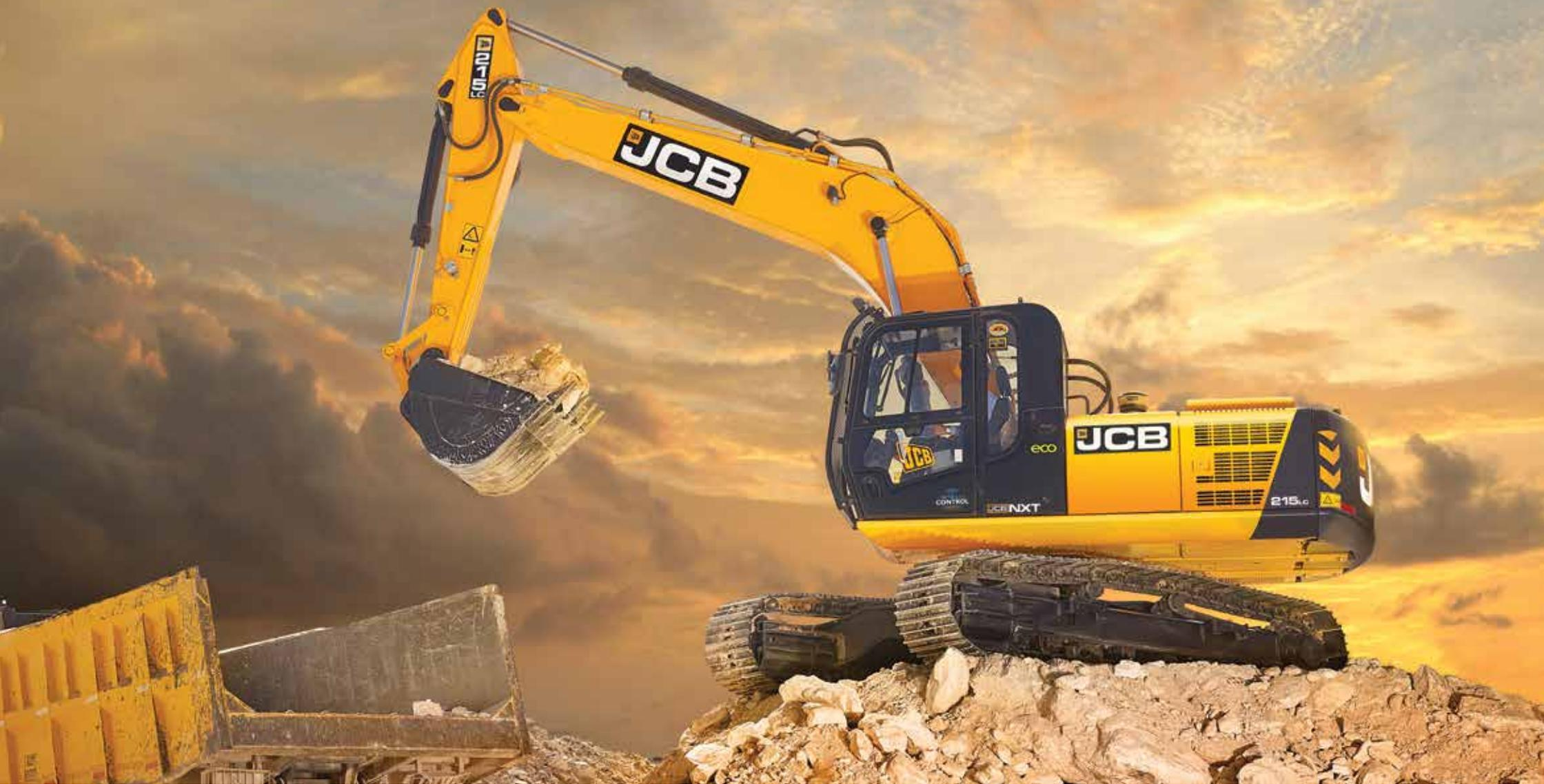
Gross engine power : 104 KW (140 hp), Bucket capacity : 0.8 cu.m - 1.02 cu.m
