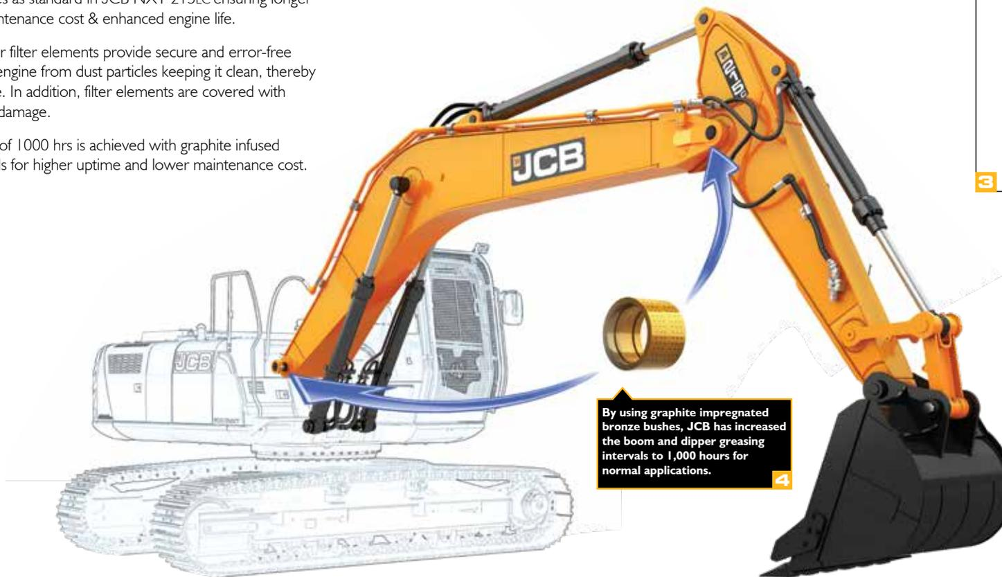
By using graphite impregnated bronze bushes, JCB has increased the boom and dipper greasing intervals to 1,000 hours for normal applications.
