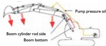
Boom, arm and bucket regeneration for faster operation and fuel saving.
