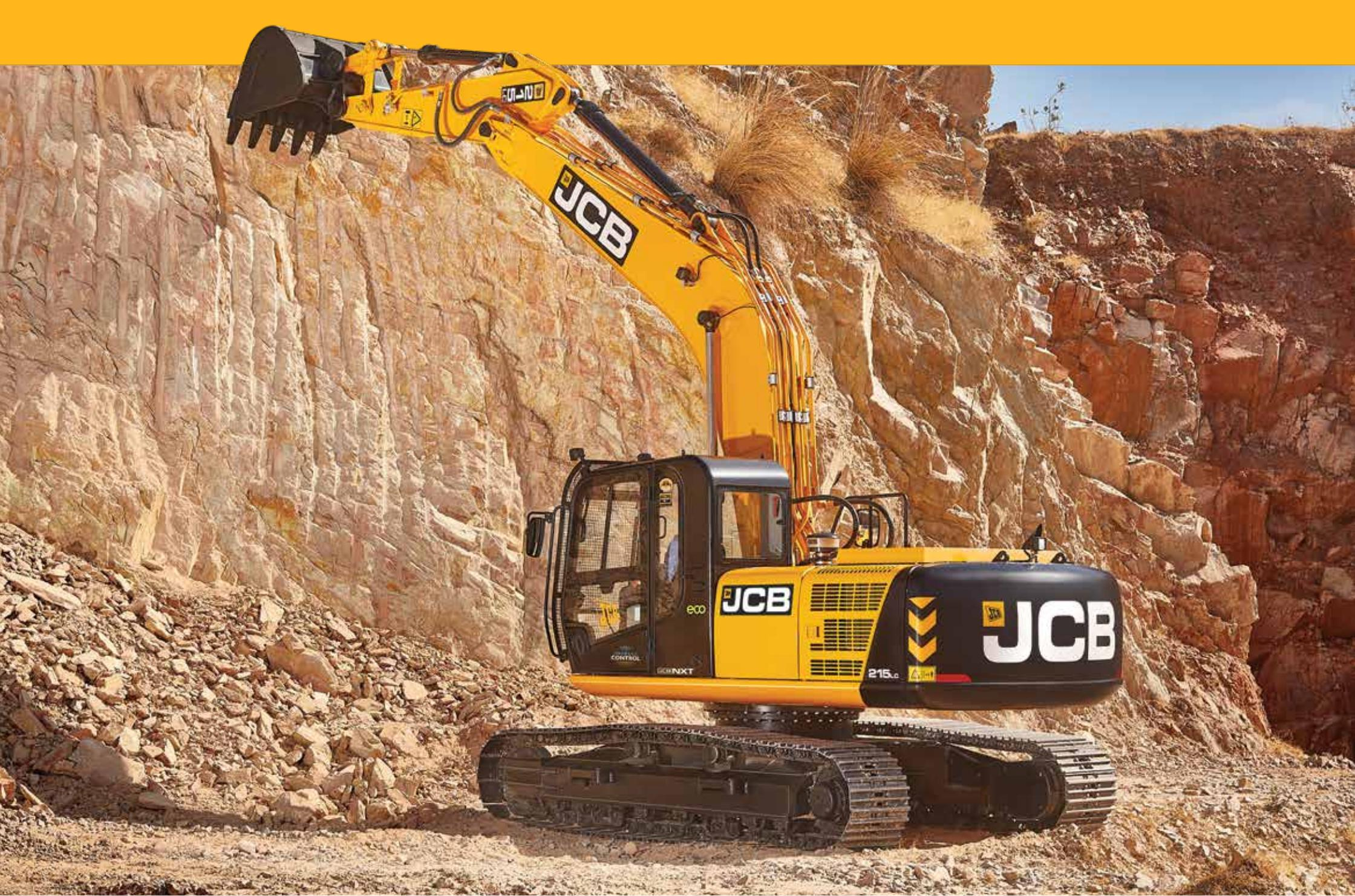
**9** 5 working lights 2 on the cab front top, 1 on boom's left side, 1 in tool box and 1 on counter weight, provide better illumination and help the operator to work efficiently even at night.
