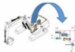
Control valve with in-built flow summation for fast & efficient combined operations.
