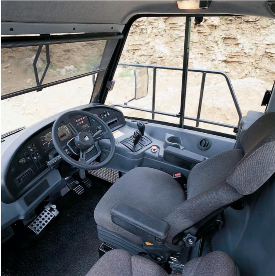
**Ride Comfort.** The three-point front suspension with its oscillating axle and low pressure ride struts, combined with the new center-mounted cab, offers unrivaled levels of ride comfort for the operator in all driving conditions. Operators remain comfortable and productive throughout the day.
