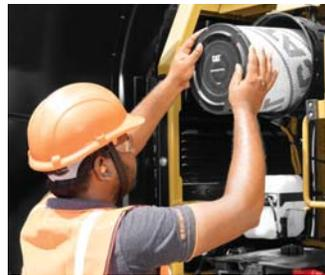
RADIAL SEAL ENGINE AIR FILTER
