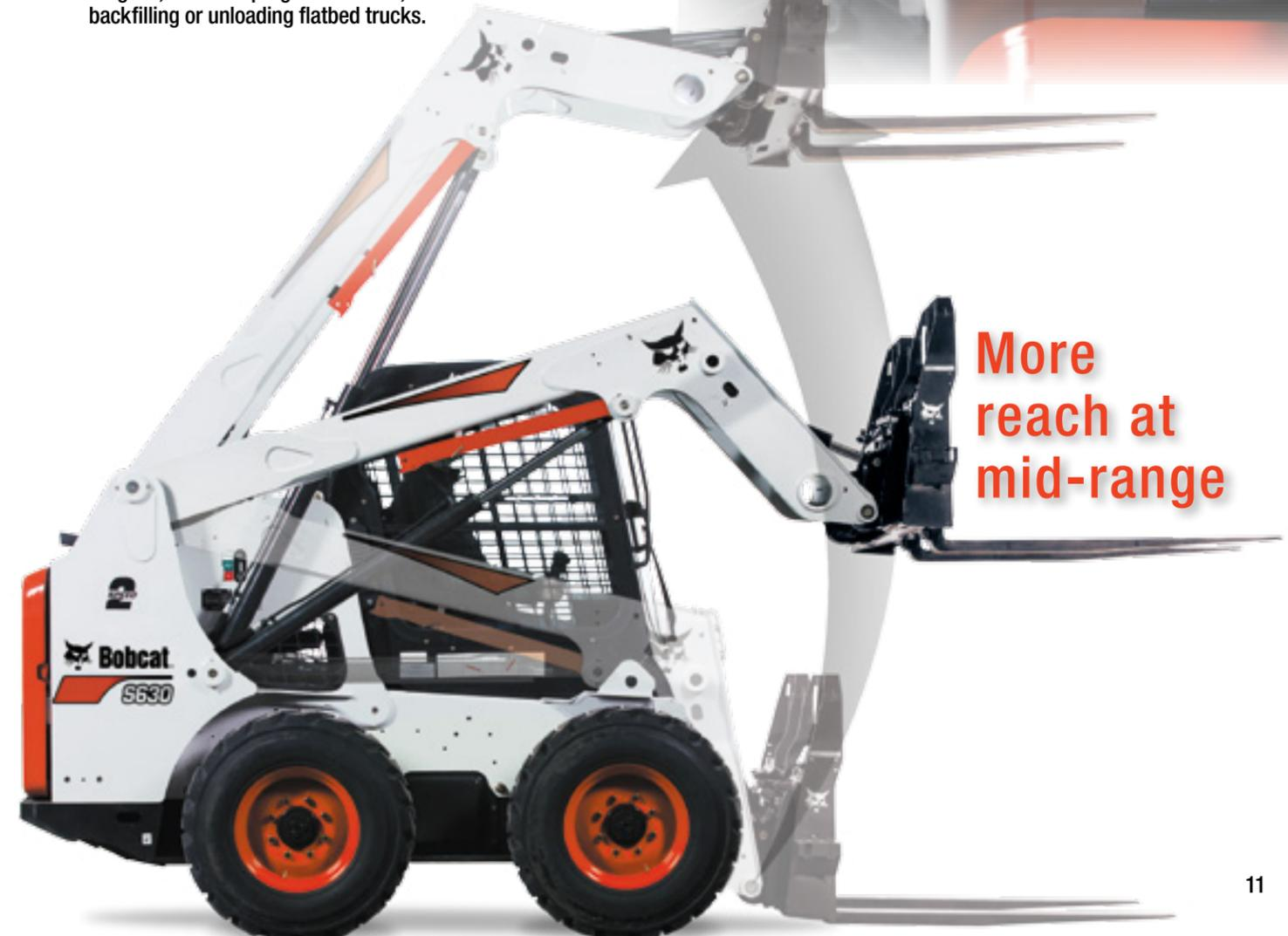
Every pin and connecting point on Bobcat lift arms are part of a single-plane design. Side-to-side movement is minimized, resulting in less wear and longer life. It also helps prevent unwanted spillage of material.
