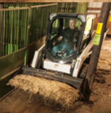
The skid-steer loader can pivot 360 degrees, which makes it one of the most maneuverable pieces of equipment available.
