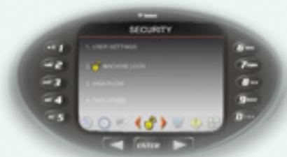
**Functional Lockouts** Protect your investment from misuse or accidental use by locking out certain functions such as high-flow hydraulics and 2-Speed travel.
